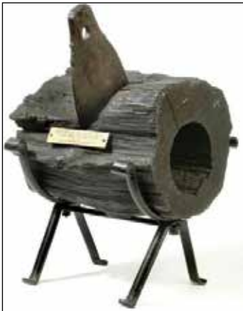
Figure 3. Section of New York City water pipe made of Atlantic white cedar, 1800-1840. This section of pipe was installed by the Manhattan Water Company, founded in 1799. The company was originally envisioned by public officials as a provider of pure waters from north of the city. The company's goals were never realized – its only source was a modest existing well near the Collect pond, the mostly wooden mains reached only a portion of the city's residents, and the water quality was often poor. Image © New-York Historical Society. [Overall: 24 × 15 × 15 in.; Gift of Mr. J. W. Rutherford, 1907].
